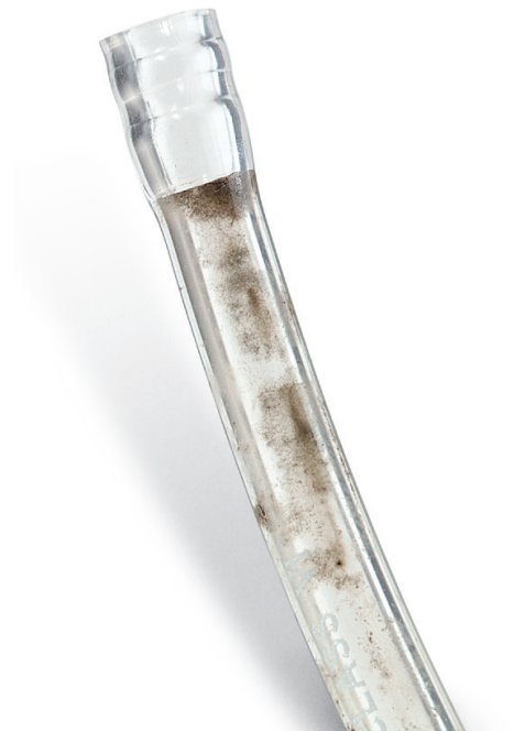
Microbial growth in wash system tube; could affect plate washing and increase background or generate unexpected results.
