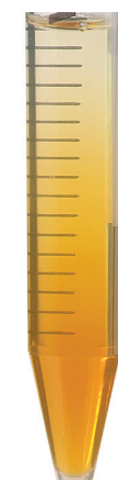
Unmixed thawed sample; proteins settled on bottom of tube; mix prior to taking sample.
