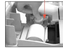
Figure 2: Install the new pump cartridge and then push down the pump roller
